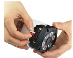
Fig.2 Remove screws and insert SD card
