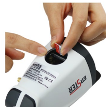
Fig.1 Remove the rubber cover and insert SD card
