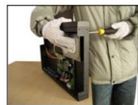
③fix the screw of hard disk
