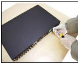
①disassemble the screw
