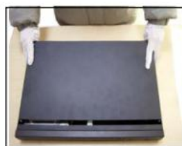
②disassemble the cover
